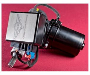
The EZ power steering unit is compact and either sits under the dash, or in the case of a LHD 911, in the 'smuggler's box' in the front luggage area. The steering can be set up for differing levels of assistance
