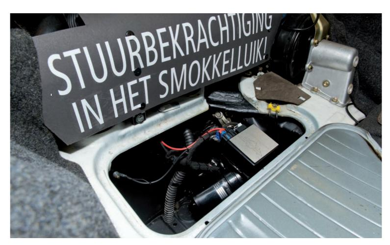
the factory-option Behr air con system from 1970. The smuggler's box was originally designed into the 901 shell as a more central location for the battery, but fortuitously it now provides a home for EZ to stash their electronics.
