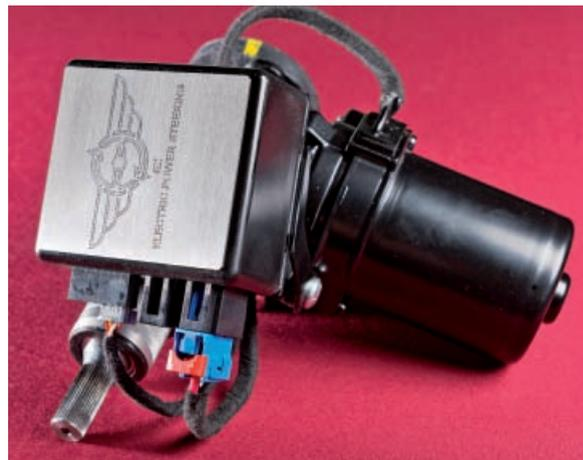
*On RHD cars, the 'smuggler's' box is much smaller, so EZ locates the kit on the second steering column shaft. The 'black box' contains the electronics which control the level of servo-assistance*
